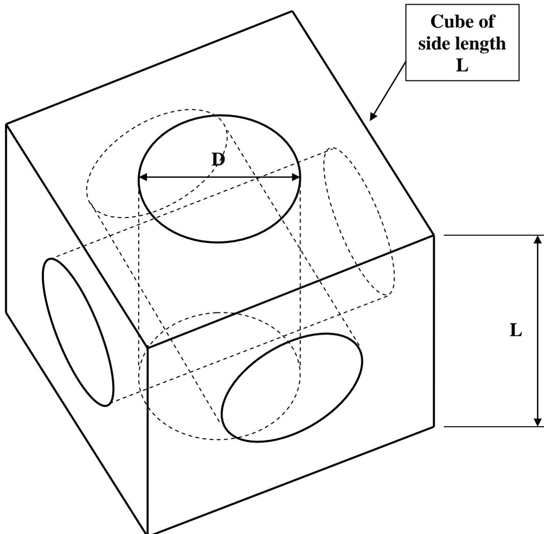
The above sketch represents a schematic view of the cube with three mutually perpendicular holes drilled through, but not showing any internal detail of the three intersecting holes.
