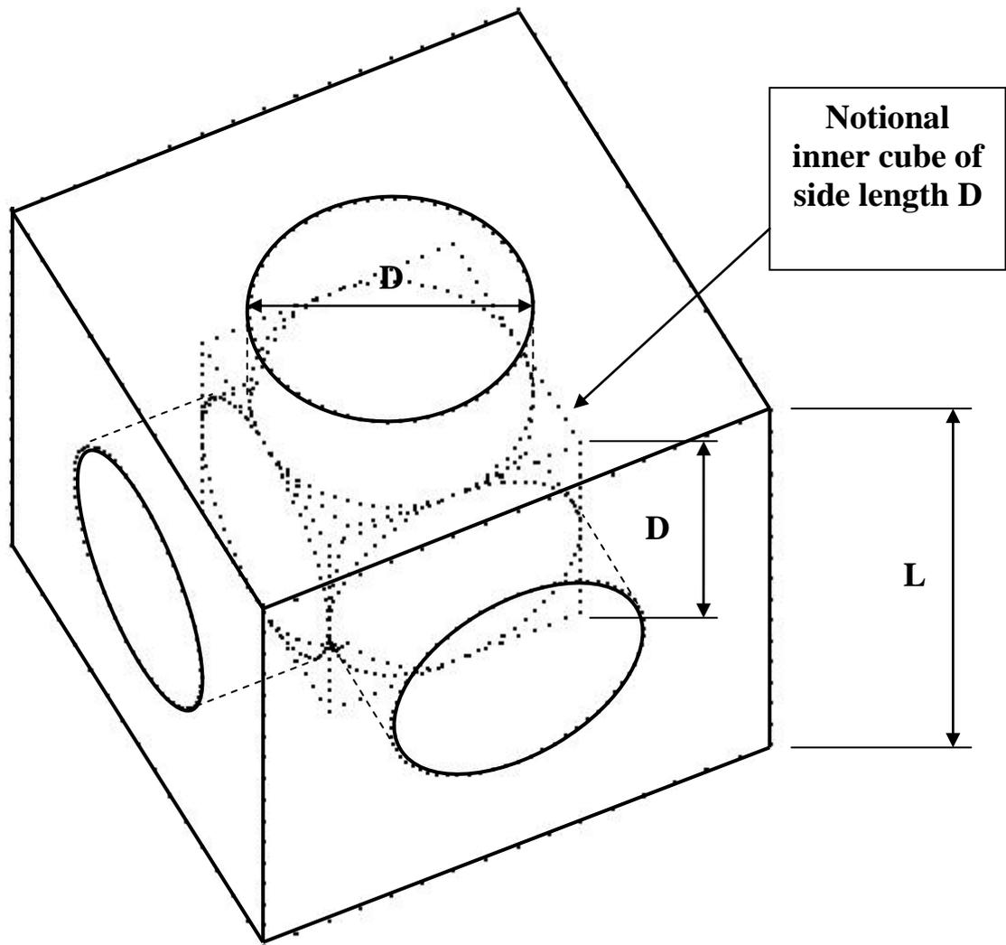
**From the above sketch, it can be seen that the intersection zone of the three drilled holes can be considered to be bounded by a notional inner cube of side length  $D$ .**
